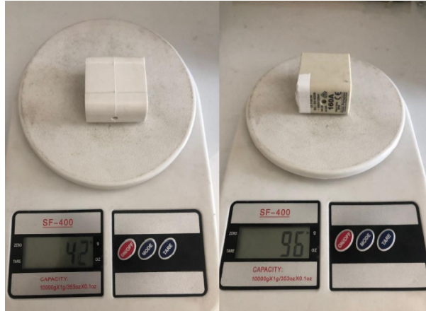
Figure 17 Comparison of Polymer Thermoset Body and Porcelain Body
