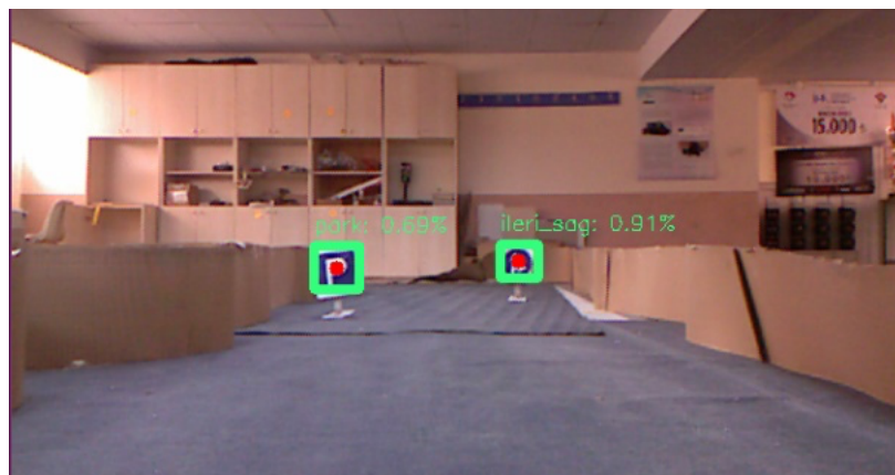
Figure 10. Autonomous movement of the robot in case of no data loss
