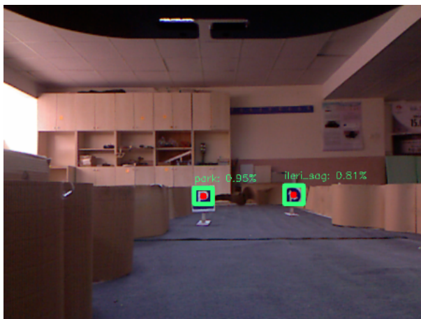
Figure 13. According to the traffic signs, the robot moves along the left-hand parking plate
